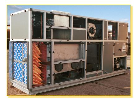
The smallest AHU is  $4000L \times 1150W \times 2150H$  supplied split into 3 sections for handling purpose with overall weight 2000 kg.
