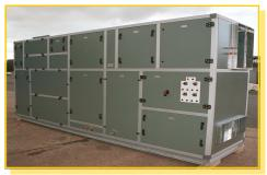
Additional cooling is provided by a single stage of DX refrigeration with the circuit fully factory piped inside the AHU using R407C refrigerant. The condenser coil, for heat rejection is located in the exhaust airstream.
